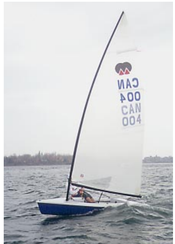
Below: A flexible mast, perfectly matched to the sail, provides maximum drive for heavy crews yet is easily de-powered in a breeze whether the boat is being sailed by two or singlehanded.
