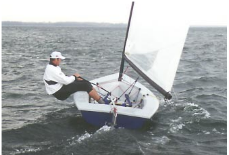
Above: The boat has a huge two person cockpit. The sides of the cockpit are taken down to the hull so there is no false bottom. This makes the cockpit very deep for the big person who then does not have to sit with knees up under the chin! Standard with every boat are toe straps fitted in the crew area, forward of the traveller.
